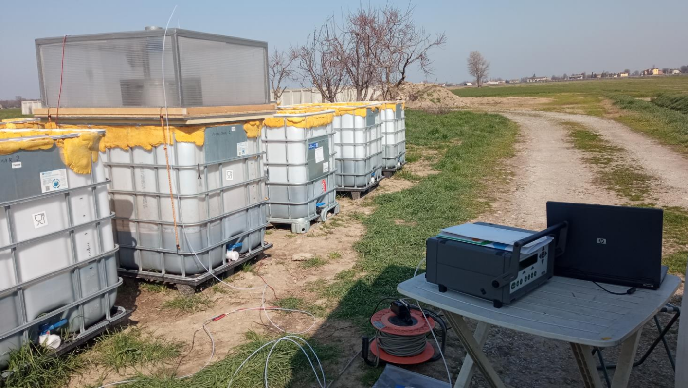
Static chamber method (Brewer et al., 1999; Hornig et al, 1999; Pedersen et al., 2001)
